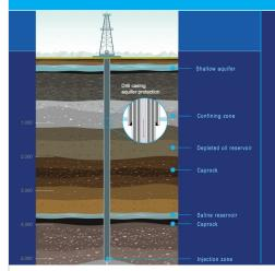
The wellbore's injection casing was cemented with  $CO_2$ resistant cement across the injection zone in guidance with EPA requirements if the wellbore becomes a  $CO_2$  injection well.
